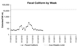
In December, all permit conditions for Fecal Coliform were met. Fecal Coliform is an indicator of the presence of pathogens. The levels of these bacteria after disinfection show how effectively the plant is inactivating many forms of disease-causing microorganisms.
