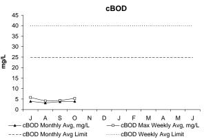
In October, both the weekly and monthly concentrations of cBOD were well below permit limits. cBOD, or Carbonaceous Biochemical Oxygen Demand, is a measure of the amount of dissolved oxygen required for the decomposition of organic materials in the environment.
