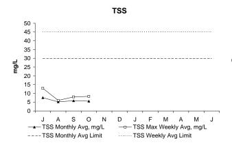
In October, both the weekly and monthly concentrations of TSS were below permit limits. TSS, or Total Suspended Solids in the effluent, is a measure of the amount of solids that remain suspended after treatment.
