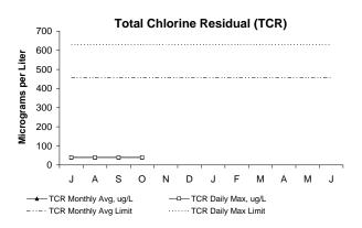
In October, both the maximum daily and monthly concentrations of TCR were below permit limits. TCR, or Total Chlorine Residual in the effluent, is a measure of the amount of chlorine that remains after the disinfection/dechlorination process. If the chlorine residual in the effluent is too high, it may threaten marine organisms.
