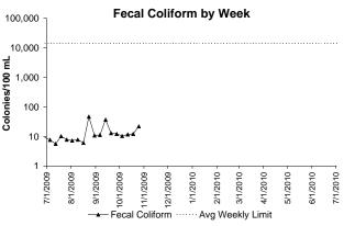
In October, all permit conditions for Fecal Coliform were met. Fecal Coliform is an indicator of the presence of pathogens. The levels of these bacteria after disinfection show how effectively the plant is inactivating many forms of disease-causing microorganisms.
