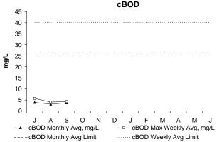
In September, both the weekly and monthly concentrations of cBOD were well below permit limits. cBOD, or Carbonaceous Biochemical Oxygen Demand, is a measure of the amount of dissolved oxygen required for the decomposition of organic materials in the environment.
