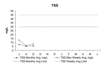
In September, both the weekly and monthly concentrations of TSS were below permit limits. TSS, or Total Suspended Solids in the effluent, is a measure of the amount of solids that remain suspended after treatment.
