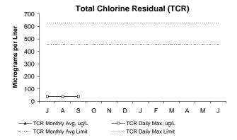
In September, both the maximum daily and monthly concentrations of TCR were below permit limits. TCR, or Total Chlorine Residual in the effluent, is a measure of the amount of chlorine that remains after the disinfection/dechlorination process. If the chlorine residual in the effluent is too high, it may threaten marine organisms.
