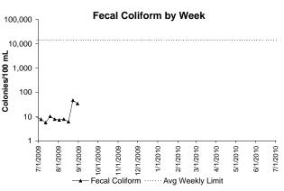
In August, all permit conditions for Fecal Coliform were met. Fecal Coliform is an indicator of the presence of pathogens. The levels of these bacteria after disinfection show how effectively the plant is inactivating many forms of disease-causing microorganisms.
