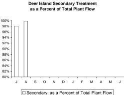
99.9% of the total plant flow to DITP was treated through secondary treatment in August. The Maximum Secondary Capacity for the entire month was 700 MGD.
