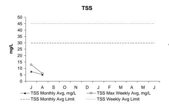
In August, both the weekly and monthly concentrations of TSS were below permit limits. TSS, or Total Suspended Solids in the effluent, is a measure of the amount of solids that remain suspended after treatment.
