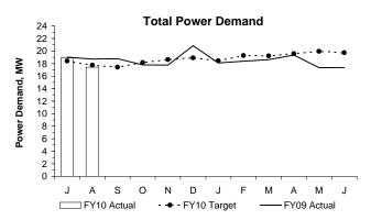
Total Power Demand for August was just under the FY10 projections by 2% even though Total Plant Flow for the month was 5% greater than the FY10 target. Power demand from total pumping alone was 5.4% higher than the FY10 projections due to above average rainfall and the subsequent higher plant flows. However, overall energy demand for most of the other treatment processes were lower than their projected targets thereby offsetting the higher than targeted power demand for pumping.
