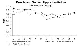
The disinfection dosing rate was 16% lower than target for August and 5% lower than the FY09 actual for the same period. The lower than expected dosage this month may be due to lower than expected chlorine demand. Chlorine demand was less than historical because the wastewater continues to contain less overall solids and organic material due to the high amount of rainfall and the resulting higher plant flow in July and August.
