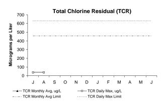
In August, both the maximum daily and monthly concentrations of TCR were below permit limits. TCR, or Total Chlorine Residual in the effluent, is a measure of the amount of chlorine that remains after the disinfection/dechlorination process. If the chlorine residual in the effluent is too high, it may threaten marine organisms.
