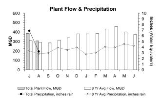
Total Plant Flow for the month of August (306 MGD) was 5% higher than the target 8-year average flow estimate for the month (291.7 MGD) as precipitation was 15% higher than the 8-year average precipitation for the month (3.24 inches actual vs. 2.82 inches expected).
