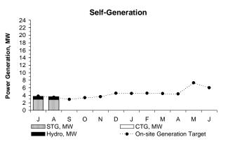
Power generated on-site was slightly above target (+5%) for August. Power generation was 3% above target by the STG and 14% above target by the Hydro turbines due to slightly higher than normal plant flows. The 0.147 MW of power generated by the CTGs was 33% higher than the 0.110 MW target due to nearly 8 hours of CTG operation during the month for a Demand Response event on August 24 and for equipment maintenance/checkout purposes (on August 18, 19, and 28).
