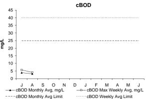
In August, both the weekly and monthly concentrations of cBOD were well below permit limits. cBOD, or Carbonaceous Biochemical Oxygen Demand, is a measure of the amount of dissolved oxygen required for the decomposition of organic materials in the environment.
