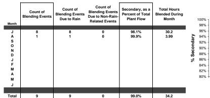
99.9% of all flows were treated at full secondary for the month of August as there was only one (1) blending event, on August 29, with 3.99 hours of blending and 14.0 Mgal of flow blended with secondary effluent. This blending event was triggered by the 1.65 inches of rain that fell, as a tropical depression passed offshore, and the resulting high plant flows. **Secondary permit limits were met at all times.**
