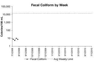
In July, all permit conditions for Fecal Coliform were met. Fecal Coliform is an indicator of the presence of pathogens. The levels of these bacteria after disinfection show how effectively the plant is inactivating many forms of disease-causing microorganisms.
