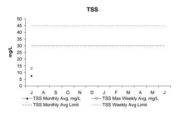
In July, both the weekly and monthly concentrations of TSS were below permit limits. TSS, or Total Suspended Solids in the effluent, is a measure of the amount of solids that remain suspended after treatment.
