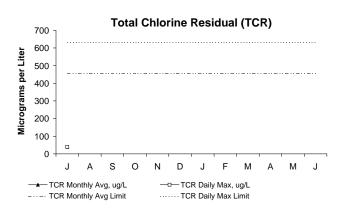
In July, both the maximum daily and monthly concentrations of TCR were below permit limits. TCR, or Total Chlorine Residual in the effluent, is a measure of the amount of chlorine that remains after the disinfection/dechlorination process. If the chlorine residual in the effluent is too high, it may threaten marine organisms.
