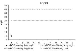
In July, both the weekly and monthly concentrations of cBOD were well below permit limits. cBOD, or Carbonaceous Biochemical Oxygen Demand, is a measure of the amount of dissolved oxygen required for the decomposition of organic materials in the environment.
