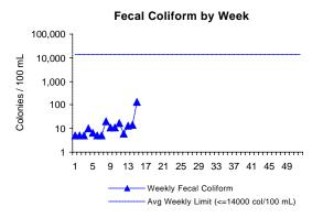
Fecal Coliform is an indicator of the presence of pathogens. The levels of these bacteria after disinfection show how effectively the plant is inactivating many forms of disease-causing microorganisms. There are four conditions in the permit including daily geomean, a weekly geomean, 10% of all samples, and three consecutive samples not to exceed 14000 col/100mL. In September, all of these conditions were met.
