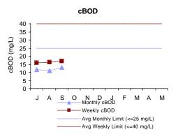
The cBOD is a measure of the amount of dissolved oxygen required for the decomposition of organic materials in the environment. In September, both the weekly and monthly concentrations were well below permit limits. The 5-day cBOD removal rate for September was 88.3%.
