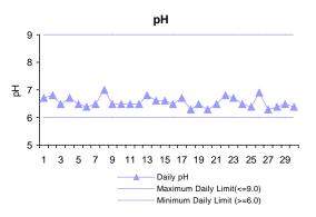
pH is a measure of the alkalinity or acidity of the effluent. Sudden change in pH does not have an adverse effect on marine environments. Because of the pure oxygen used in the activated sludge reactor, the effluent pH tend to be at the lower pH range. In September, all pH measurements were within the permit limit range.
