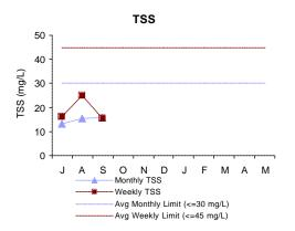
Total Suspended Solids in the effluent is a measure of the amount of solids that remain suspended after treatment. In September, both the weekly and monthly concentrations were well below permit limits. The TSS removal rate was 90.3%.
