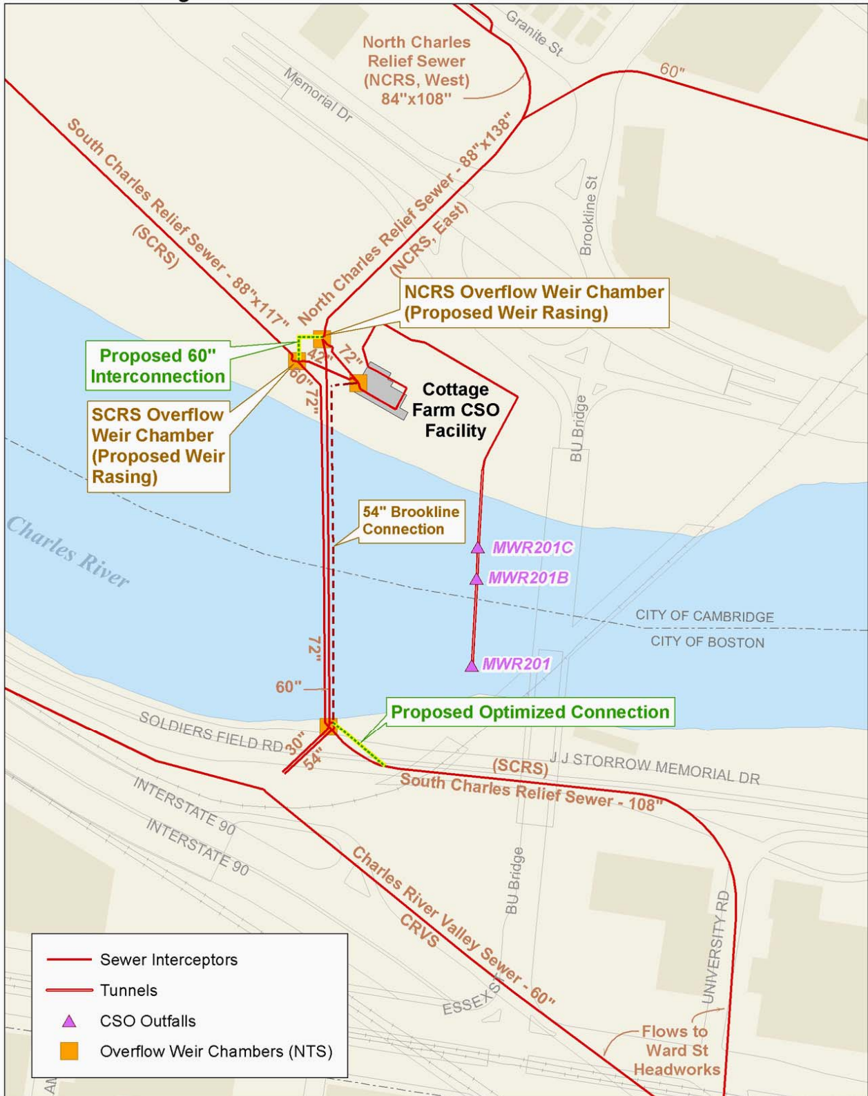
Figure 8 Cottage Farm Brookline Connection and Inflow Controls
